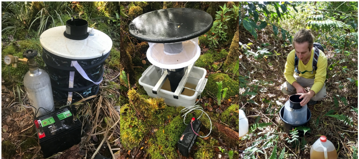
Figure 2. Traps used for mosquito surveys. From left to right: BioGents CO 2 traps (targets females seeking blood meals); active CDC gravid trap (targets females seeking oviposition sites); passive GAT gravid trap (also targets females seeking to oviposit).
